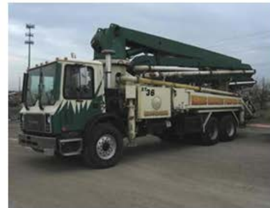
Concrete Pump Truck
