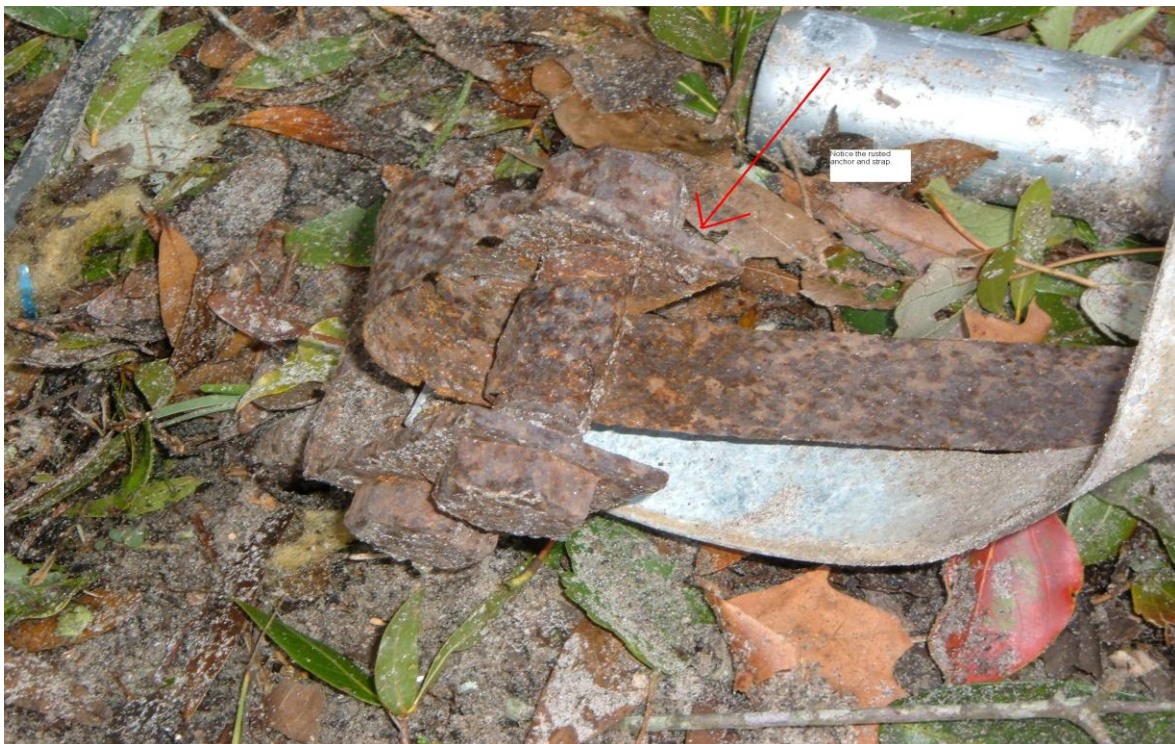
These pictures show the rusted anchors and straps that failed to keep the home from going airborne and moving from its foundation.
