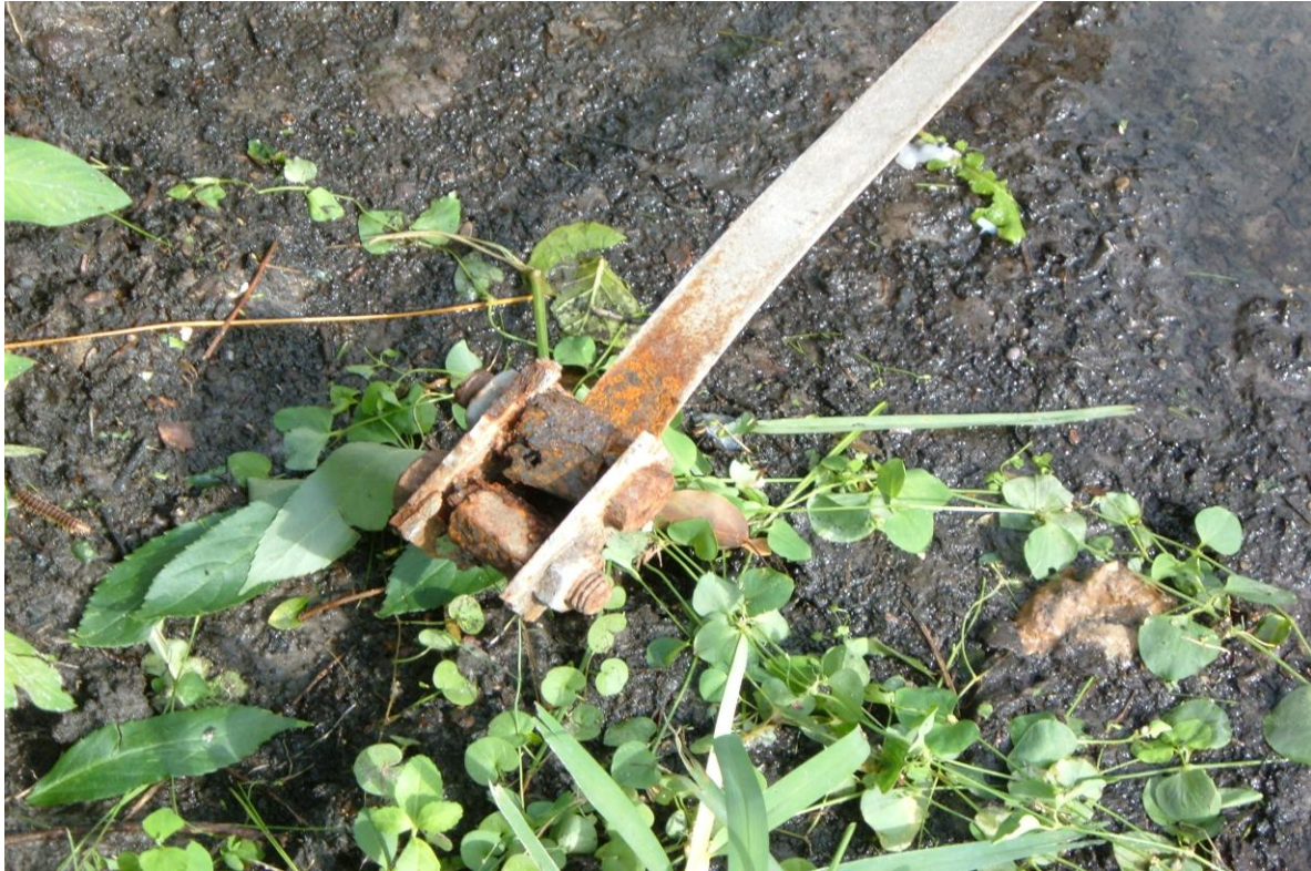
These pictures show the rusted anchors and straps that failed to keep the home from going airborne and moving from its foundation.
